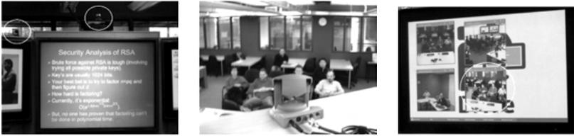
**Figure 4.** Central rear-projected display, with two mounted front-view cameras (top, cameras circled), with view from behind the left-camera (bottom-left image), and video-feed of left-camera (circled in bottom-right).
