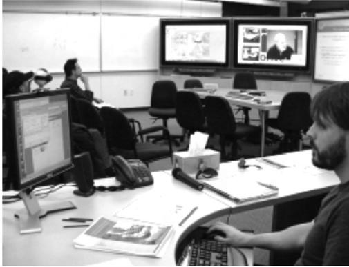
**Figure 6.** Desk of Technical Supervisor for D-Drive, located to the right of the display environment, with contact with Technical Supervisors for all of the remote sites via messaging software on the desktop machine.
